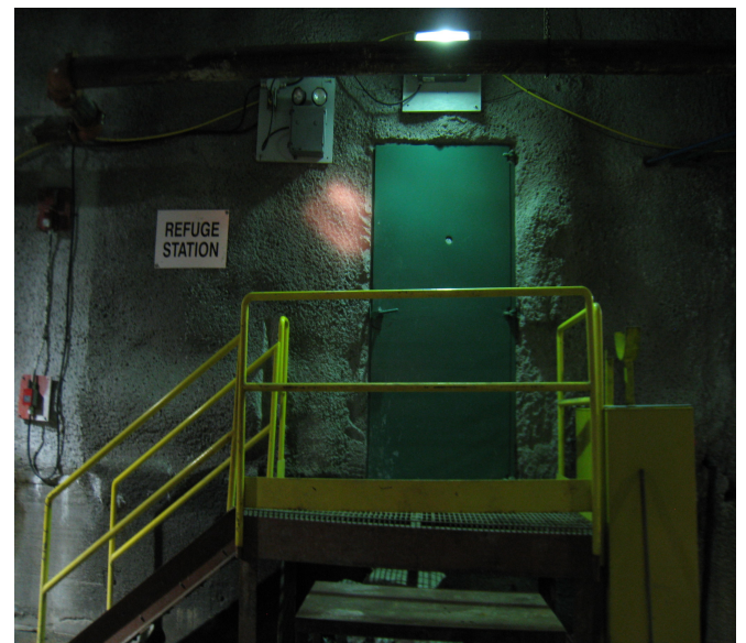
FIGURE 7 REFUGE STATION AIRLOCK
